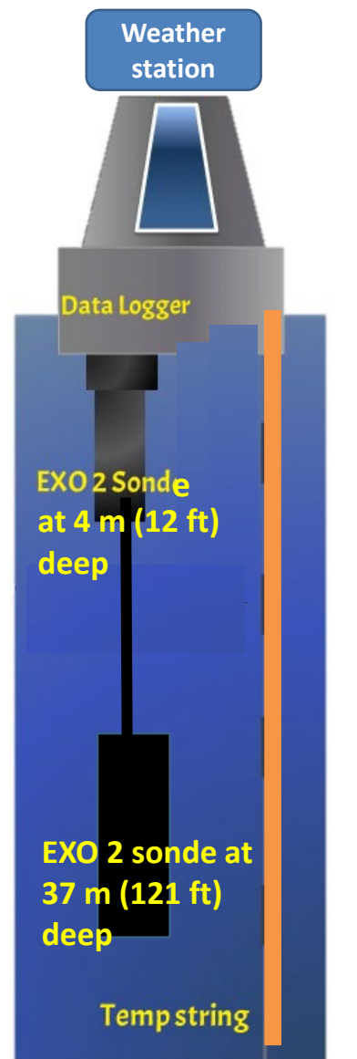
EXO 2 sonde with multiple probes for different water quality parameters
