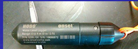
HOBO Data Logger Measure Stage
