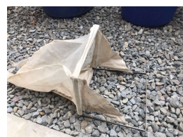
Figure 1. Image of 1ft 3 Surber sampler used in this experiment
