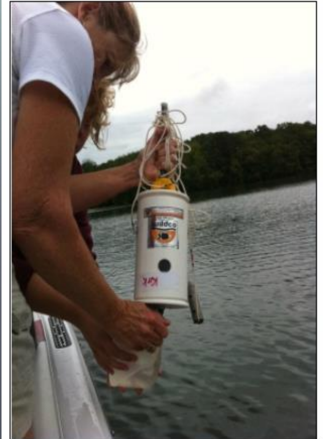
CSLAP volunteer collecting water sample with Kemmerer sampler on Kirk Lake.
